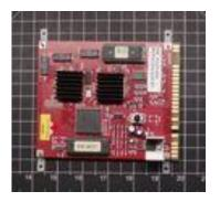
The most important and influential of these new standards was the pcb standard pinout. Any game pcb complying with that pinout standard is what we now call a JAMMA board.
